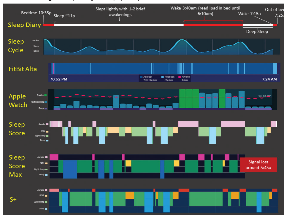
Figure 1 —Comparison of overnight sleep diary data (top row) to data from six CSTs that were simultaneously collected.
