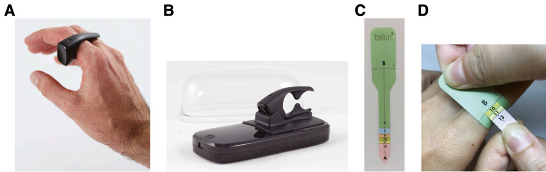
(A) Belun Ring securely worn on the proximal phalanx of the index finger; (B) Belun Ring sitting on the charging cradle; (C) Paper ring selector; (D) Measuring finger size with the paper ring selector.
